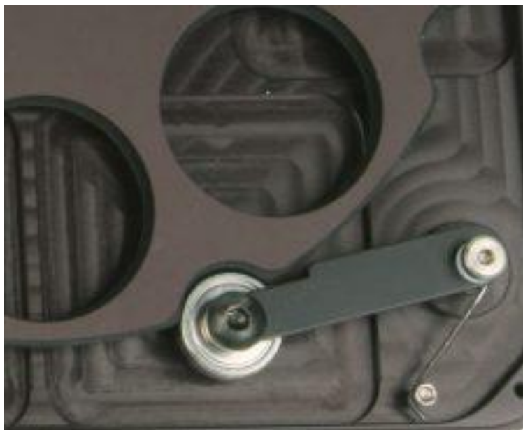
Positive detent mechanism provides single-pixel filter position accuracy
